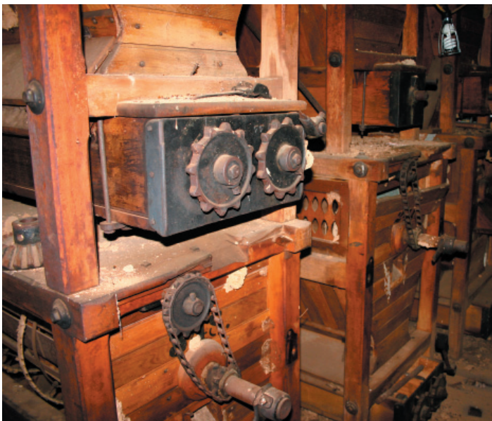
FIGURE 1-14. Sifting and grading machines survive on the third story, arrayed along the eastern side of the room and fed by grain delivered from below by canvas conveyor belts enclosed in wooden housings and powered by a drive shaft at tie-beam level.
