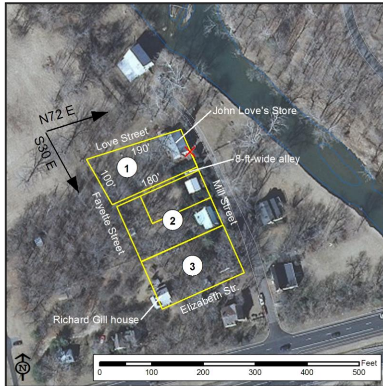
Figure 101: GIS map showing the proposed reconstruction of the boundaries of Lot 1 and overlaid on recent aerial photography. Note the rotations of the western and northern sides of Lot 1 relative to Lots 2 and 3 to the south.
